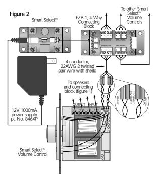
**NOTE:** The EZB-1 and EZB-2 connecting blocks have connectors that are labeled L+, L-, R-, R+. You will need to make connections to the connecting block using alias names (i.e. 12v=L+, Gnd1=L-, Gnd2=R-, Data=R+).
